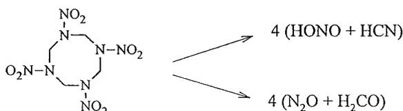
**Figure 2.** Decomposition pathway of HMX (ref 7).
